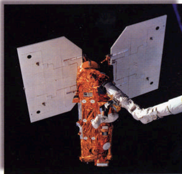
ERBS was the first Ball and GSFC satellite deployed by the shuttle arm.
